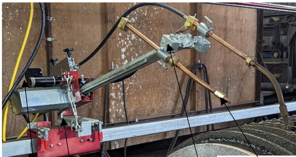
Opening Style Carriage for ease of assembly Zinc plated steel beam Sealed motors with encoders Flexible torch mounting
