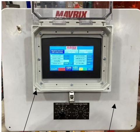
Polycarbonate protective cover Durable Light Weight Fiberglass Enclosure
